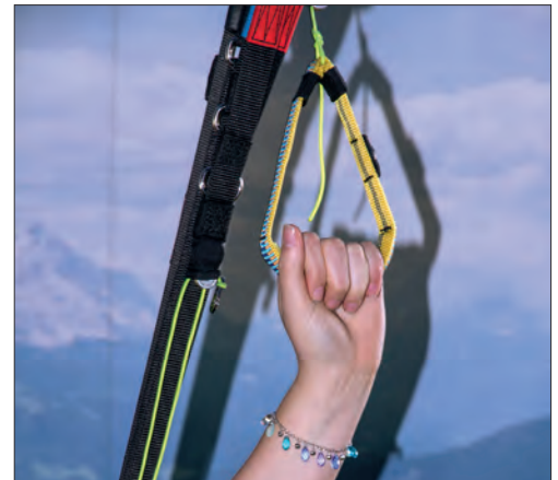
Figure 15: This position of the brake handle is recommended for beginners and should be chosen when manoeuvres are flown with an increased angle of attack (Big Ears, B-Stall). • Photo: Papillon
