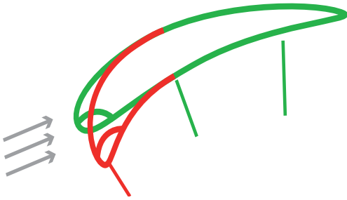
Figure 48: Risk of frontal collapses when the air strikes from above
