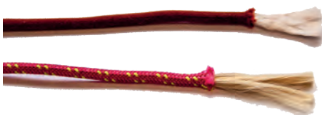
Figure 13: Aramid (top) and Dyneema (bottom) lines
