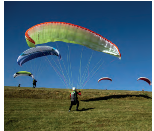
Figure 19: Ground handling training with Mike Küng, Wasserkuppe. It is useful to practice the full stall during ground handling to learn how it feels. In the air the still safe minimum speed is reached with an approximate brake pull of 50%. Except when the canopy dives forward, there is no reason to pull the brakes more than that during the flight. The only time you use full brakes is for the landing. Photo: Papillon
