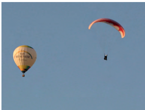
Figure 36: Aerodynamic heavier-than-air flight with a paraglider. By contrast, hot-air balloons use the principles of aerostatics. • Photo: Papillon
