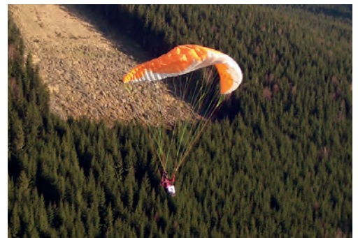
Figure 17: A provoked collapse for demonstration. With a 50% collapse like here the wing can still be flown straight and would allow a “standing” touchdown. Collapses like this are extremely rare with EN-A wings and only occur in severe turbulence. Photo: Markus Fiedler
