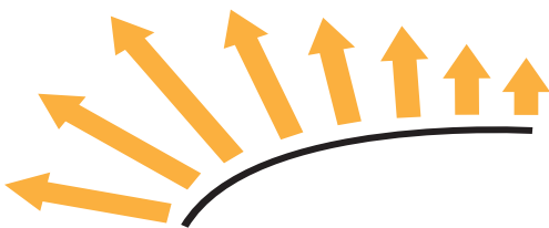
Figure 50: Suction effect / negative pressure at the upper surface of the wing
