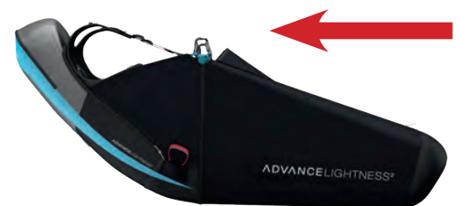
Figure 22: Low carabiner suspension: more sensitive to control inputs by weight shifting, requires experience Example: Advance Lightness 2
