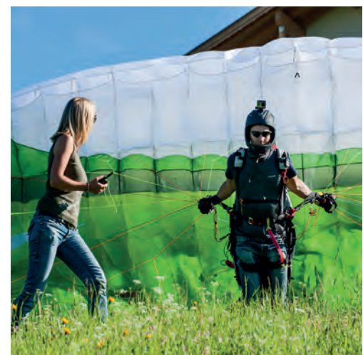
Figure 8: During the launch air enters through cell openings at the leading edge of the canopy and inflates it • Photo: Felix Wölk
