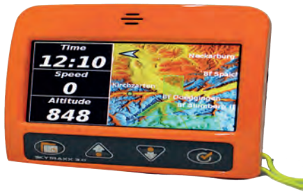
Figure 27: High-end variometer with GPS from Skytraxx
