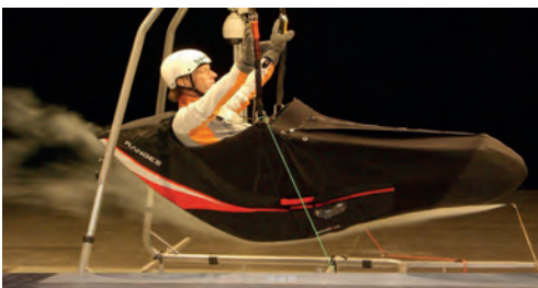
Figure 58: Skywalk optimises harnesses in the wind tunnel • Photo: Skywalk
