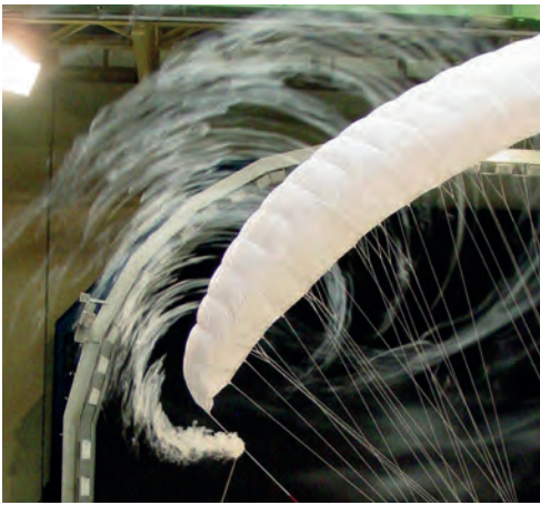
Figure 56: Smoke used to make the wake vortex of a paraglider wing visible • Photo: Skywalk
